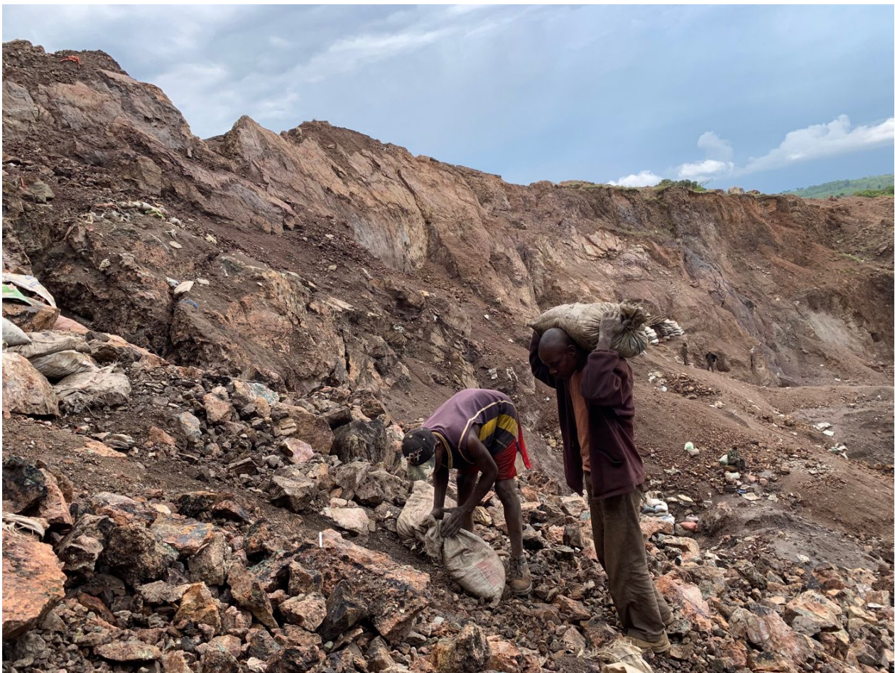
Artisanal cobalt miners working with hand tools in an open pit in the Democratic Republic of the Congo.
